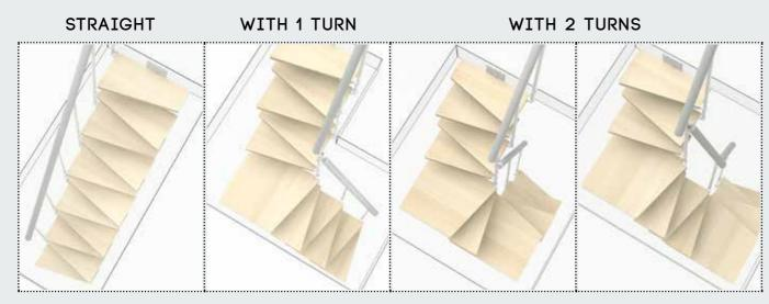
STAGGERED AND SHAPED STEPS: reduce the space occupied by the staircase without sacrificing comfort.
